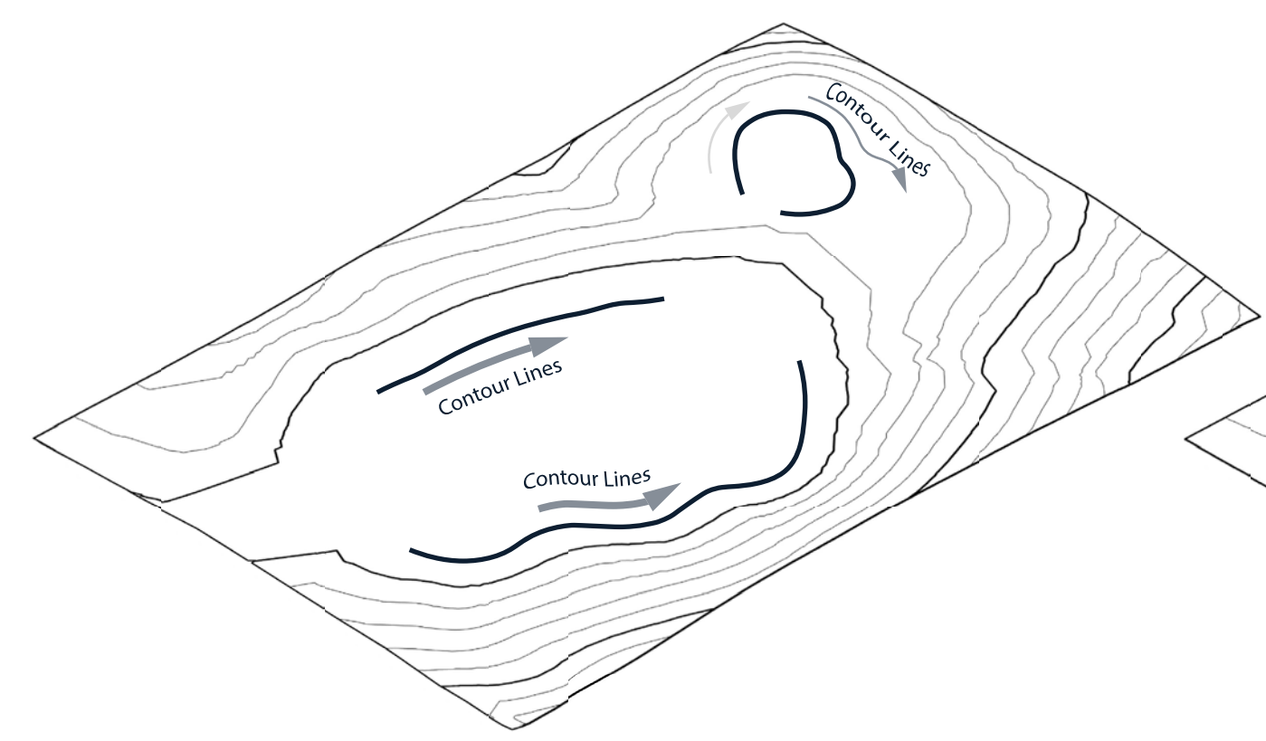
The contour of the educational complex repeats the interpolation contour of the slope due to which we can have one level for the whole area.
